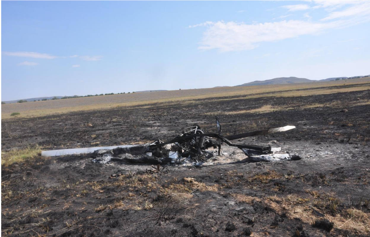
Figure 1: Wreckage as found at the accident site after been consumed and destroyed by post impact fire.
